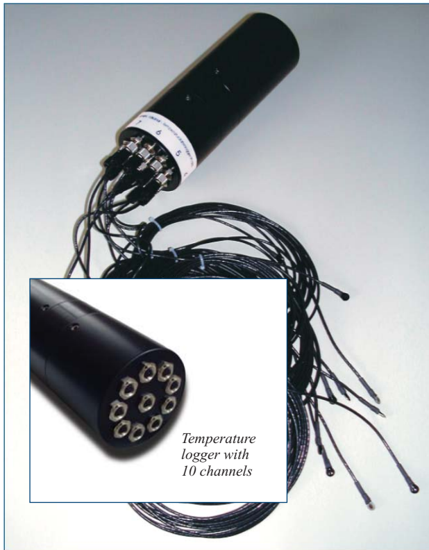
DK8010 e.g. with 10 probes for surface temperature
