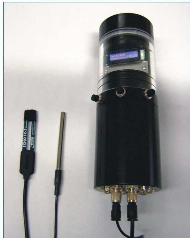
DK8015 with 5 channels for soil moisture and temperature
