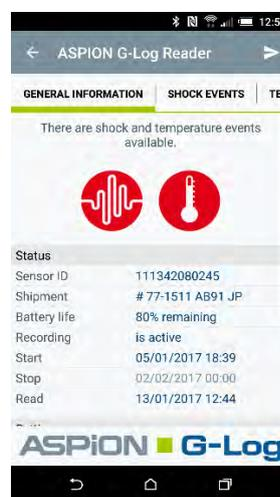
Read sensor: place your smartphone close to the sensor in the NFC chip area
