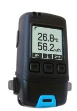
The GFX-TH standalone USB data logger measures and stores up to 252,928 temperature and humidity readings over a -30 to +80°C (-22 to 176°F) and 0 to 100%RH range at a resolution of 0.1°C and 0.1%RH.
