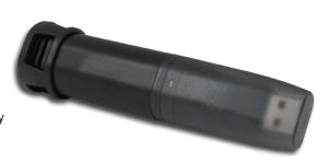
This standalone data logger measures and stores over 16,000 temperature and humidity readings from -35 to  $+80^{\circ}$ C (-31 to  $+176^{\circ}$ F) and 0 to 100%RH range at a resolution of 0.5°C (1°F) and 0.5%RH.
