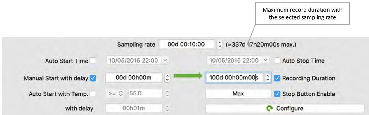
In this example, the logger will start manually by pressing the start button without any delay. The sampling rate is 10 minutes and the logger will stop automatically after 100 days.
