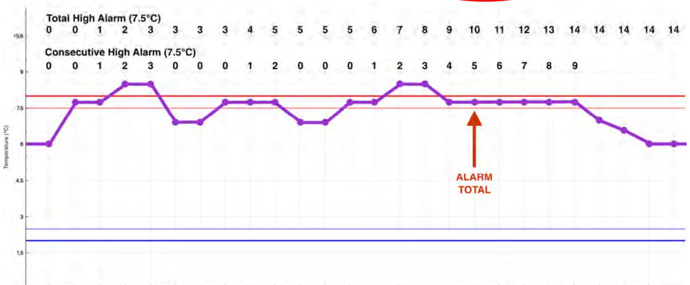
Example for a high alarm threshold set to 7.5°C with a total delay of 10 minutes and no consecutive delay. The sampling rate is 1 minute. The alarm is triggered when the total delay reaches 10 minutes. As we can see in this example, the counter stopped counting when the temperature goes back below 7.5°C and continues when above 7.5°C.
