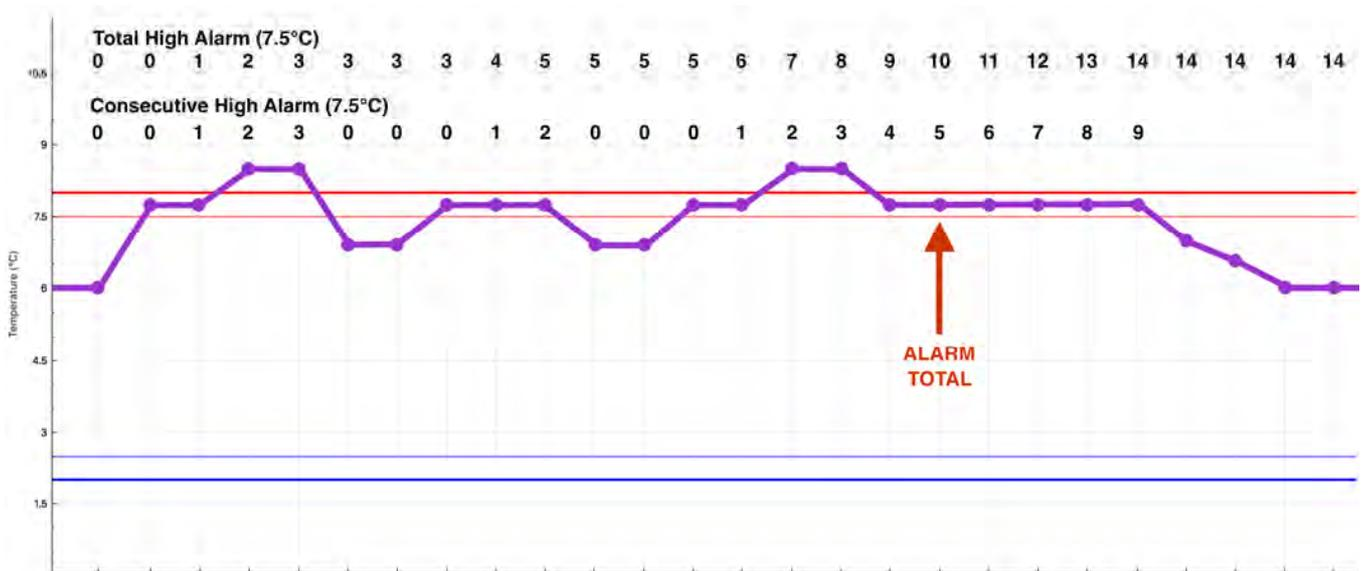
Example for a high alarm threshold set to 7.5°C with a consecutive delay of 6 minutes and a total delay of 12 minutes. The sampling rate is 1 minute.
