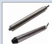
Pressure Probe PSense650 Various models as waterlevel or screw-in probes with ranges from 1 bar up to 100 bar Resolution: 0.1mm
