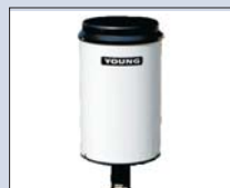
Young 52202/52203 Rain Gauge Heatable tipping bucket rain gauge, recommended by the WMO Collector surface: 200cm 2 Resolution: 0.1mm
