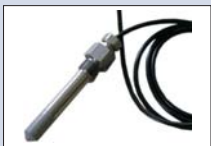
DKRF370 - Humidity/temperature probe for compressed air up to 100 bar, G3/8" thread, Operating conditions: -20...+80°C. Dimensions: 100mm x 13mm
