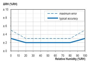
Typical accuracy of relative humidity measurements given in %RH for temperatures 0 to  $80^{\circ}$ C.
