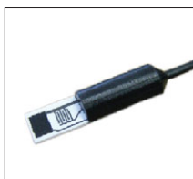
SHS-325 - Detects incipient bedewing. Signal "1" if condensation occurs, "0" if not Operating range: 0...50°C Dimensions: 43 x 10mm
